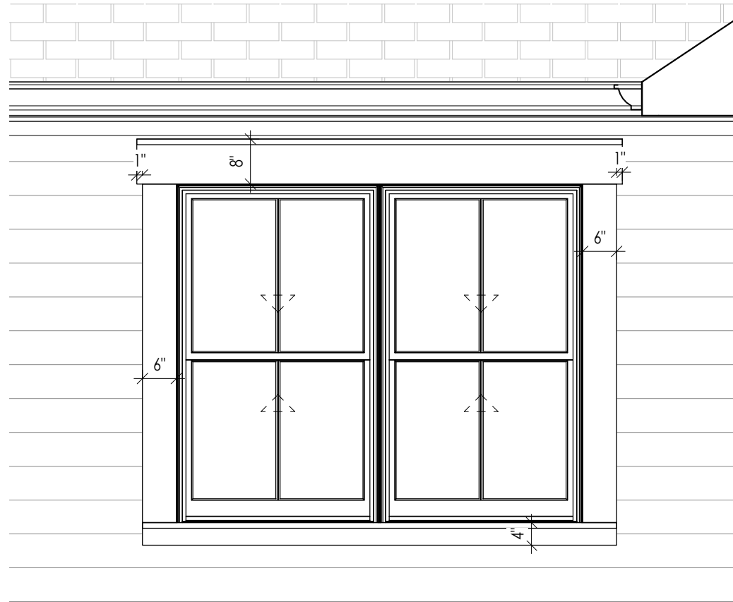
5 WINDOW TRIM ELEVATION A104 1/2" = 1'-0"
